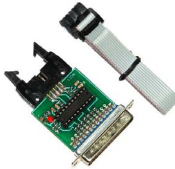
Figure 3.3: In System Programmer for AVR microcontrollers from NEX Robotics
